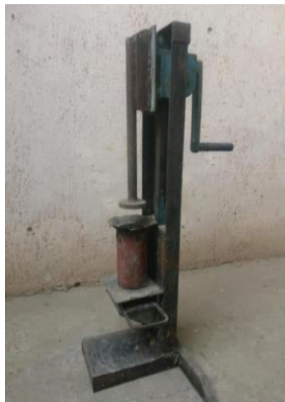
Plate 2: Locally constructed Briquetting machine (for the present work)
